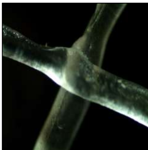
Fig. 11: Spacer after 3-hour clean with Cleaner A.
