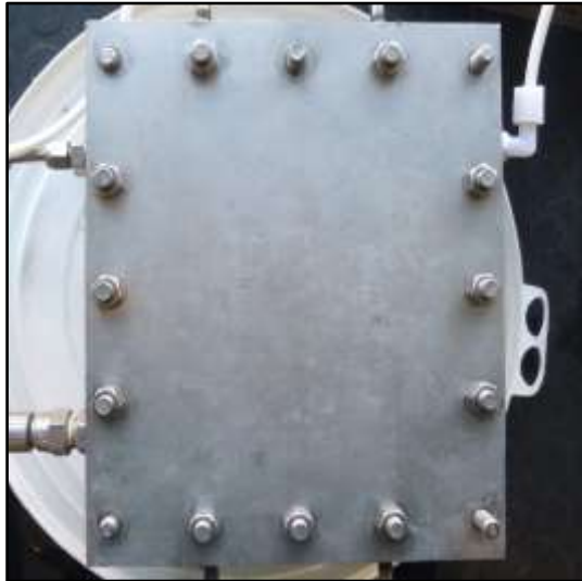
Fig. 3a: Stainless steel Flat Sheet Rig.
