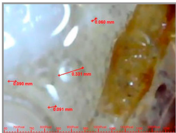
Fig. 4. Cleaner A and air creates evenly distributed microbubbles.
