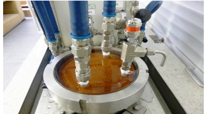
Fig 1: The Genesys flat sheet test rig (FSTR)
