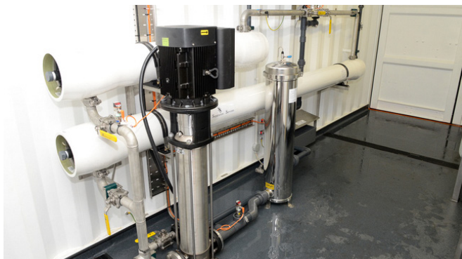
Fig 6: Genesys International pilot plant testing for membrane compatibility & cleaning efficiency of fouled membranes
