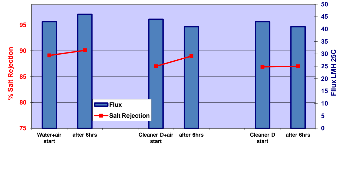
Fig 15: Compatability Performance with Virgin CA SB50 membrane
