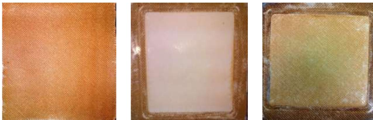
**Figure 6: Fouled membrane**
