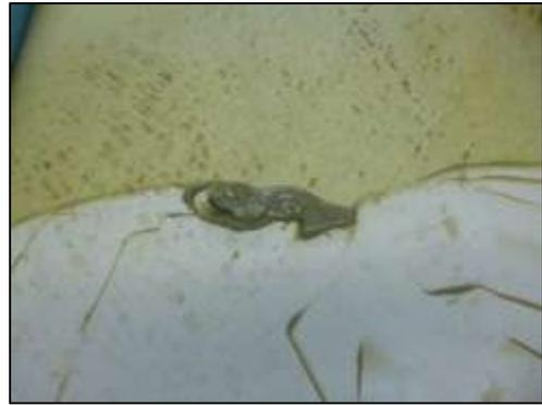
**Figure 3: Membrane fouling**
