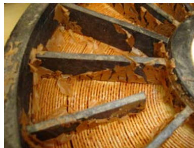
Fig 5 Iron acrylate fouling
