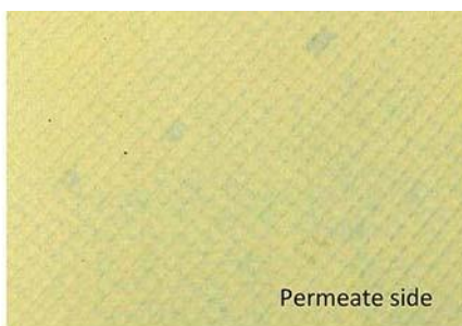
Photograph 20.- Methylene blue test positive result
