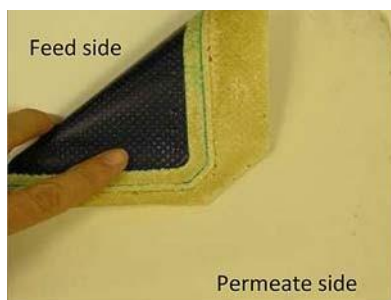
Photograph 19.- Methylene blue test negative result
