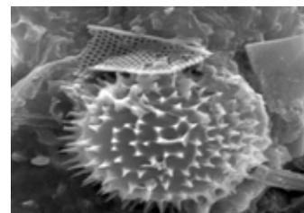
Fig 5: SEM-EDAX showing biofouling on membrane surface
