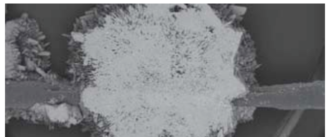
Fig 3: Rosette formation on spacer
