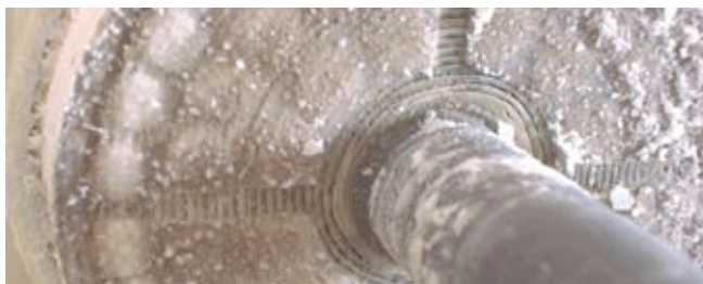
Fig 5: Calcium sulphate scale
