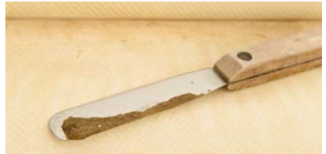
Fig 1: Clay deposit removed from membrane surface during autopsy
