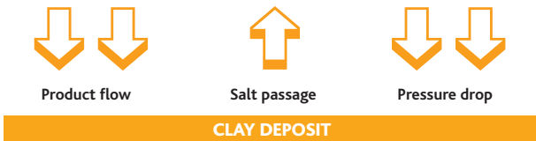
Fig 3: Effects of clay deposits on membrane performance parameters
