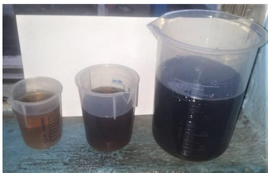
CIP Solutions after each circulation
