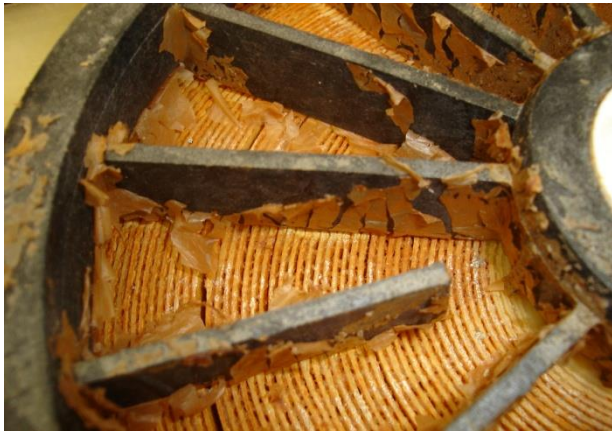
Figure 2: Iron fouling feed of a lead element
