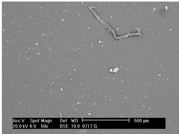
Figure 4.-SEM Micrograph. SDI membrane used for filtering 100 mL pre-treated water.
