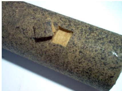
Photograph 2.-Fouling on external surface filter
