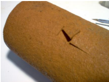
Photograph 1.-Fouling on both external and internal surfaces
