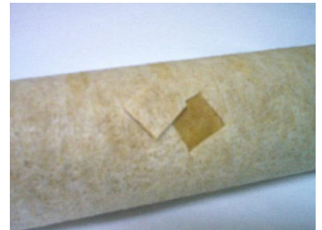
Photograph 3.-Fouling on internal surface filter
