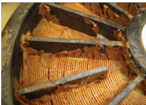
Fig. 7. Iron polymer fouling.
