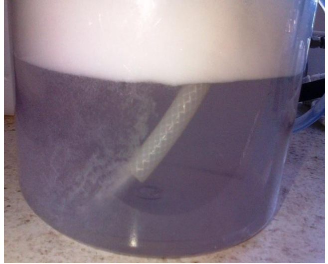
Figure 3: Air bubbles produced using proprietary cleaning chemicals
