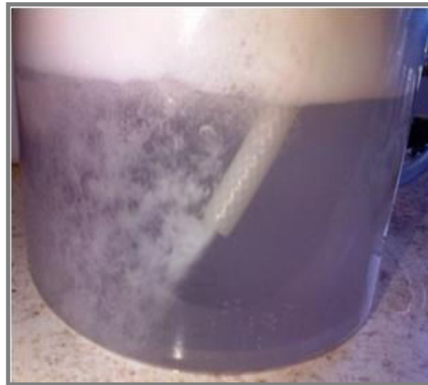
Figure 2: Small refined bubbles with air and cleaner A
