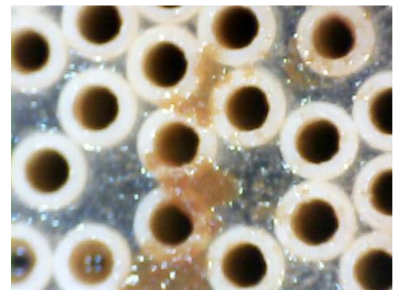
Fouling on module end
