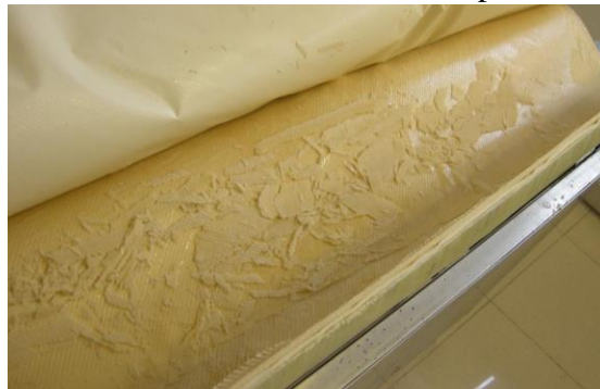
Scaling on first RO membrane position after scaled UF membrane
