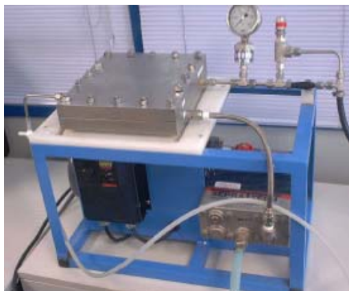
Figure 1. View of the flat sheet cleaning rig used for membrane autopsy
