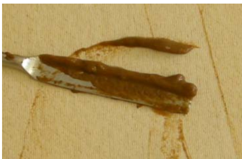
Fig 9 Clay fouling on a membrane
