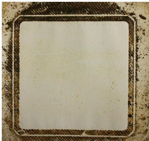
Photograph 27.- Membrane coupon after three steps cleaning (alkaline-acid-alkaline)
