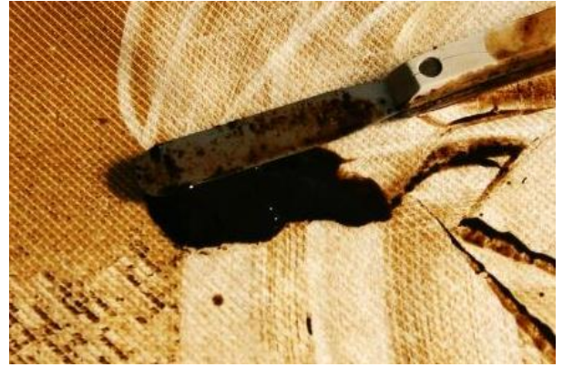
Photograph 12.- Detail of fouling with manganese: very dark brown color (MnO 2 )
