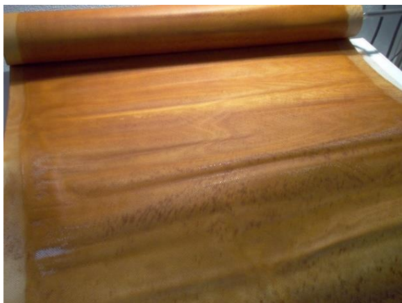
Photograph 1.- RO membrane surface with main presence of iron (as iron oxide)
