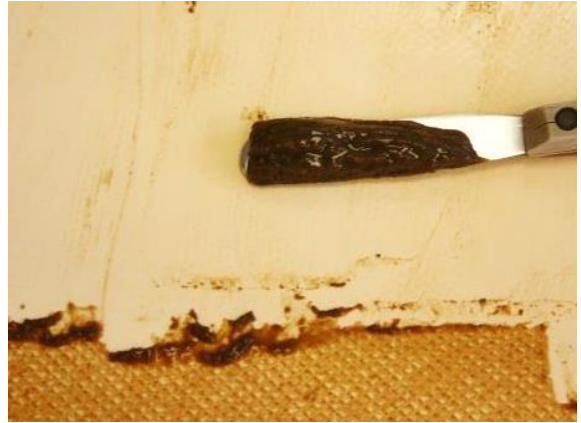
Photograph 8.- Detail of fouling with main presence of aluminium. It commonly appears mixed with organic matter and shows the color of the mixture.
