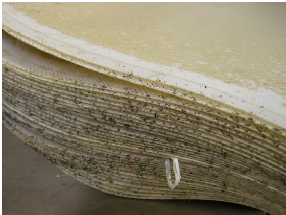
Photograph 5.- Massive presence of corrosion drags at membrane feed end
