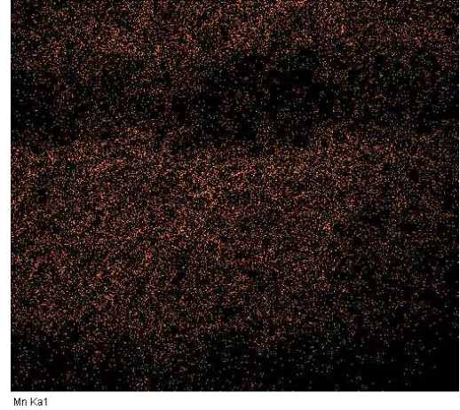
Figure 16. Distribution of manganese on membrane surface
