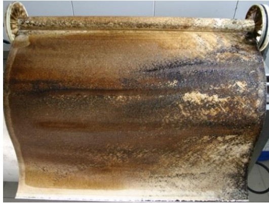
Photograph 11.- RO membrane surface with main presence of manganese fouling
