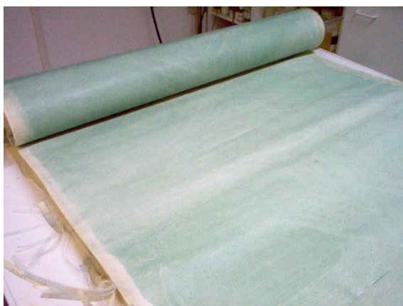
Photograph 15.- RO membrane surface with presence of chromium: green color
