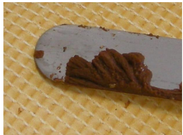
Photograph 2.- Detail of fouling with main presence of iron (iron oxide).
