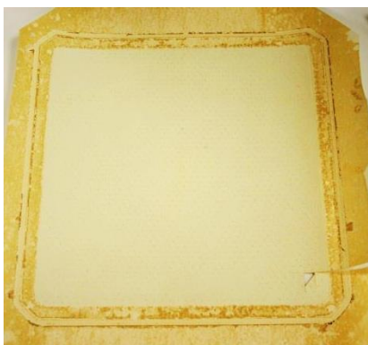
Photograph 23.- Membrane coupon after three steps cleaning (alkaline-acid-alkaline)
