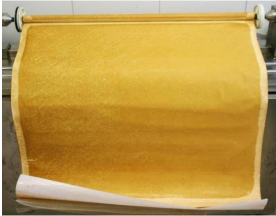
Photograph 7.- RO membrane surface with main presence of aluminium. It doesn't show any specific color different than the rest of fouling components.
