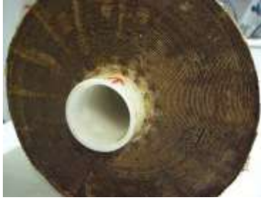
Figure 3. Deposit on feed inlet
