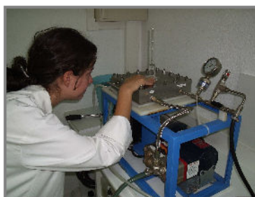
Figure 11 : Flat sheet test rig
