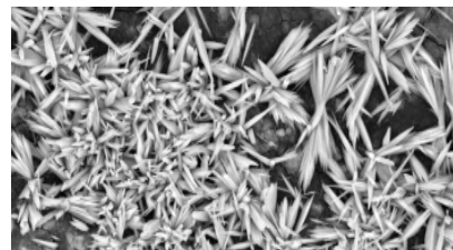
Figure 6: Barium Sulphate crystals
