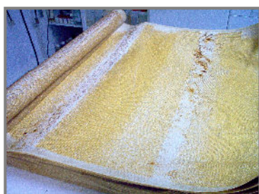
Figure 10 : clay fouled membrane
