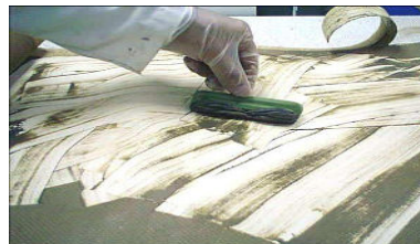
Figure 9 : clay on membrane surface
