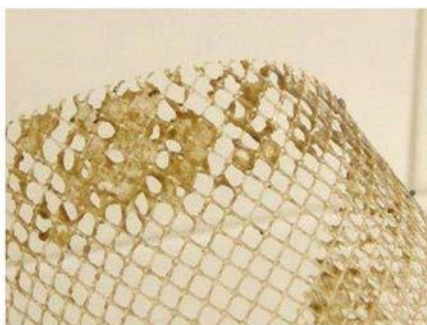
Photograph 17.- Biofouling on spacer
