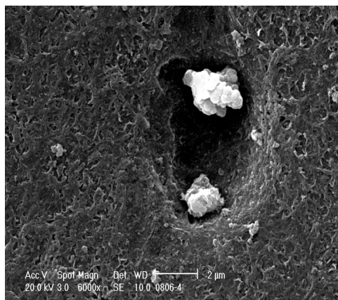
Figs. 2 and 3. SEM micrographs. Aluminosilicates and iron oxides on RO membrane surface. Abrasion process related.
