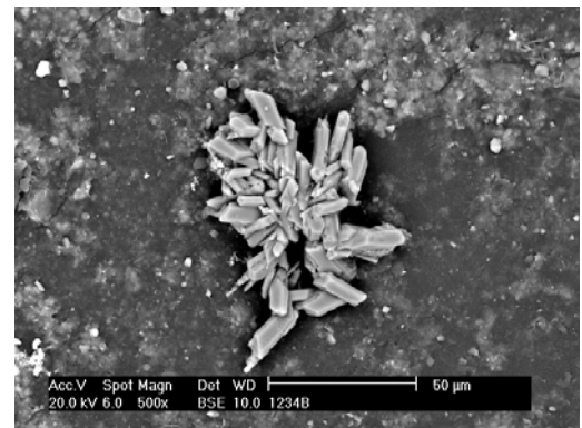
Fig 12 Calcium Sulphate scale
