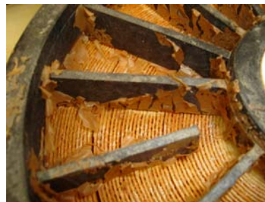
Fig 5 Iron acrylate fouling
