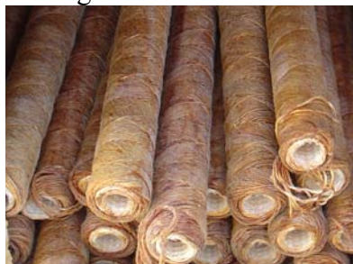
Fig 3 Iron fouled cartridge filters
