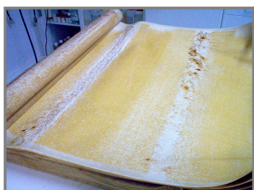
Figure 10 : clay fouled membrane
