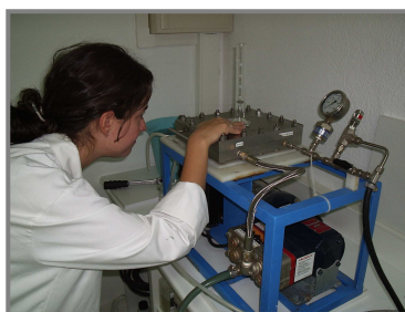
Figure 11 : Flat sheet test rig
