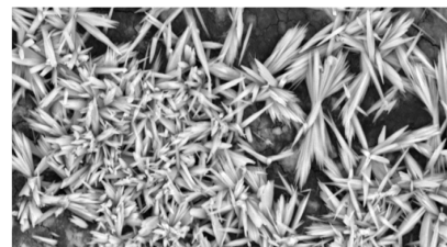
Figure 6: Barium Sulphate crystals
