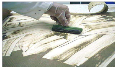
Figure 9 : clay on membrane surface
