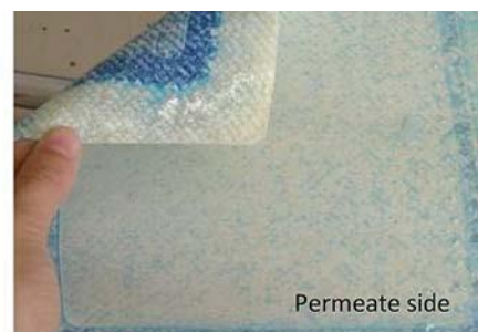
Photograph 21.- Methylene blue test massive positive result
