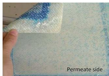
Photograph 21.- Methylene blue test massive positive result
