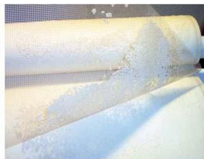
Photograph 18.- Calcium Sulphate scale on spacer
