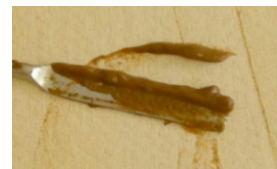
Fig 7: Clay fouling on a membrane
