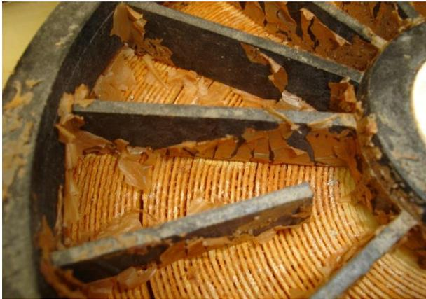
**Figure 2: Iron fouling feed of a lead element**
