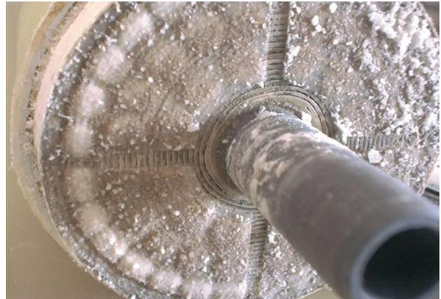
**Figure 3: Calcium sulphate last stage element**
